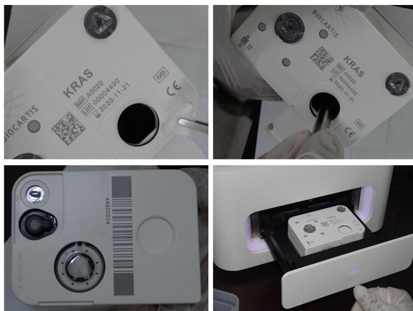
Figure 4. From left to the right, the first three pictures are demonstrating how the FFPE sample is placed inside the cartridge of Idylla™ platform. The last panel shows insertion of the cartridge into the device.
